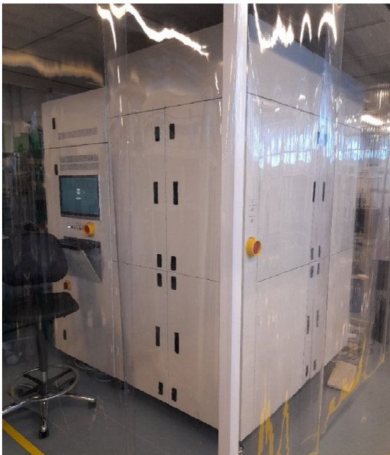
The prototype of a product for optical inspection of bonding quality and alignment measurement
