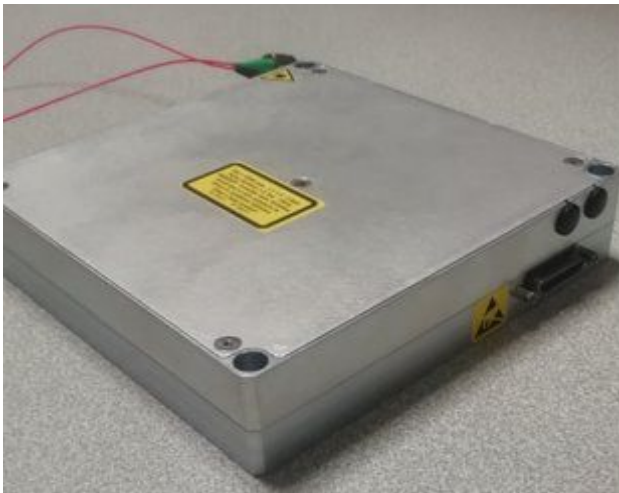
New fiber laser illuminator, as integrated in the BEAMAGINE/UPC demonstrator
