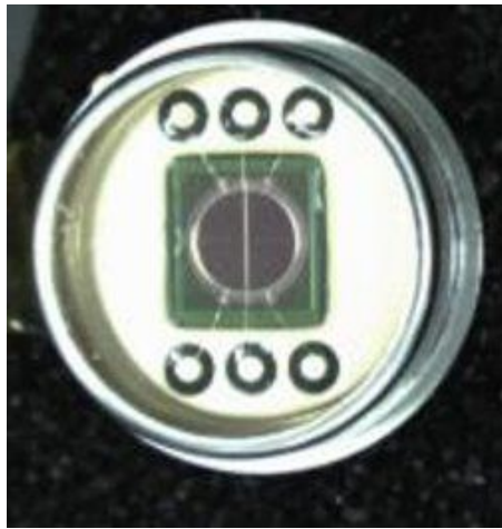
3mm diodes & 4Q integrated in TOx
