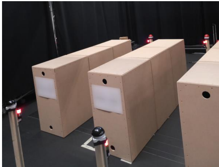
Figure 3: Picture of the demonstrator setup at [IEE] showing the simulated access control gate installed in the field of view of the camera
